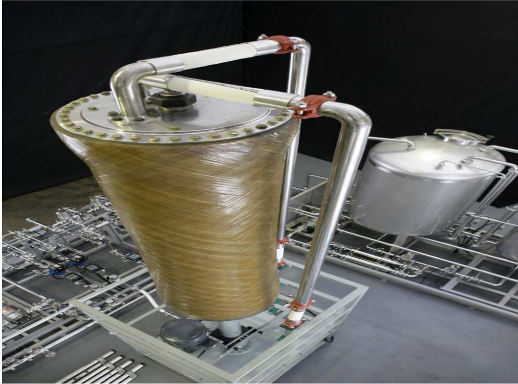
Fig.10 Wastewater Vibrating Membrane Treatment System
